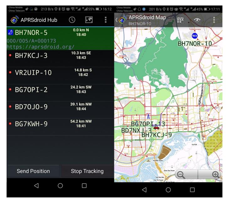
After the setting is completed, enable: start Tracking. At this time, the red indicator light inside the Bluetooth converter box is long, indicating that the APRSDROID is connected to the Bluetooth converter box. When the FT400 receives the decoded beacon, it will immediately transmit to the APRSDROID via Bluetooth. To the APRS list, you can also see the specific location or trajectory of the other party through the APRS map in real time.
