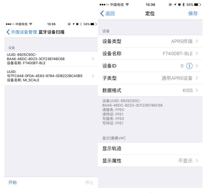
Choice: Universal APRS device, the default communication mode of the program is KISS, compatible with FT400 radio output KISS
