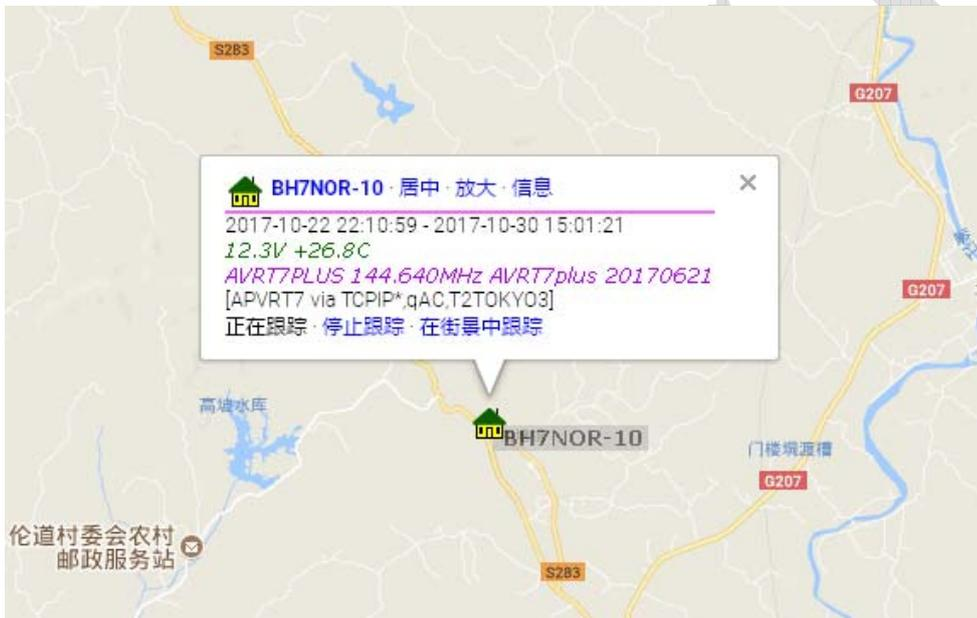
After using SHT3x, BME280, BMP180, DHT21/AM2301, AVRT7plus uploads the beacon to the APRS server and automatically converts to the weather station mode. (firmware version 20181212)
