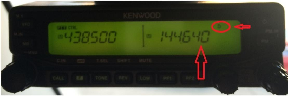
After the above settings, T6 Via **KENWOOD TM-V71A/TM-V71E** B Bands send and receive **APRS** Data, A Band can be a normal QSO.
