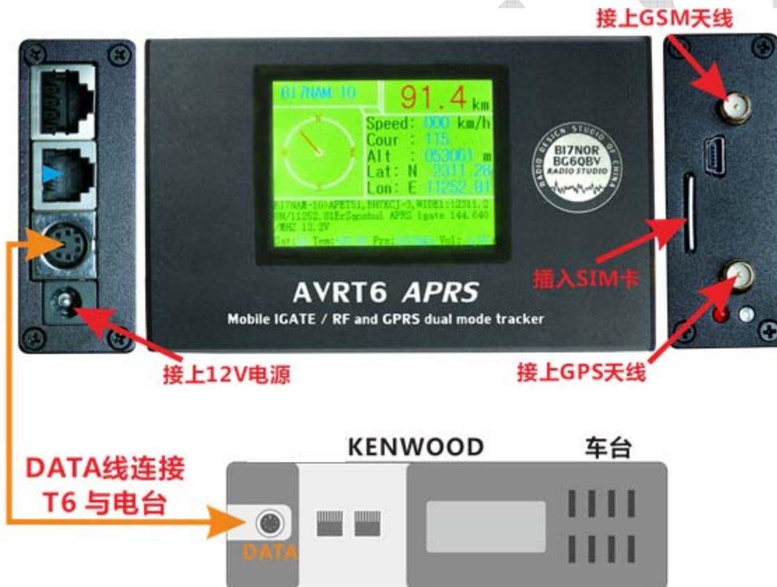
To facilitate the T6 APRS Send and receive data, simple setup will be necessary before use. Setting procedure is as follows:
