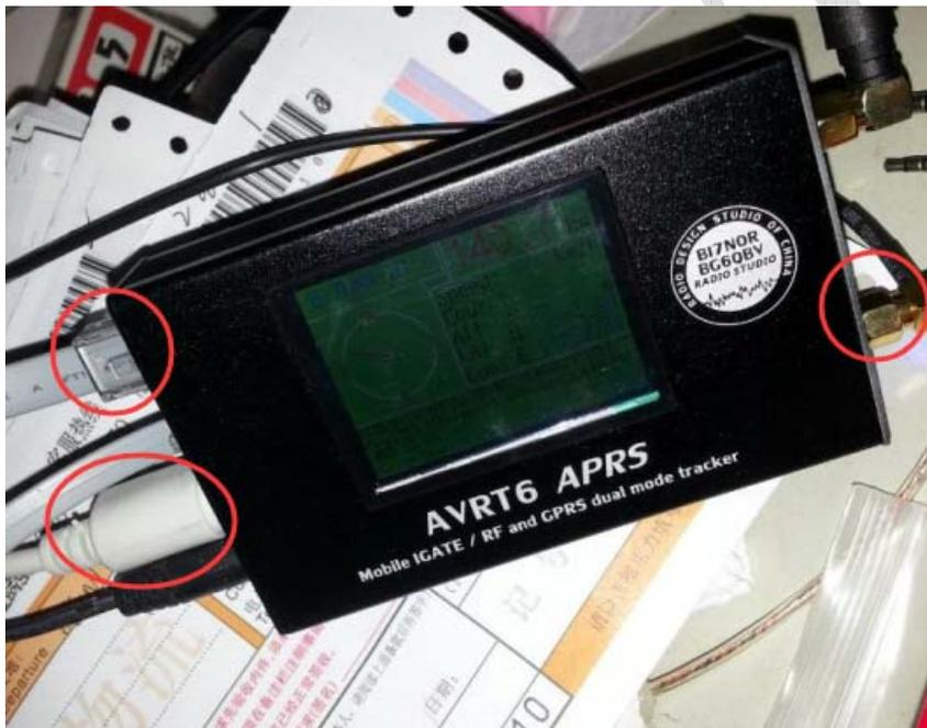
Access to the 12V power, AVRT6 will come with LED flashing on electric starter, LCD display LOGO, post fired 1 time into normal working state.
