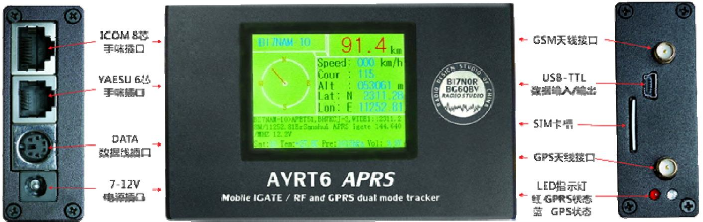
2. radio emission features: requires connection T6 DATA to radio DATA, radio microphone and microphone, as well as the T6 MIC interface are connected with links. Connect GPS antenna, you can get a job in radio APRs working mode.
