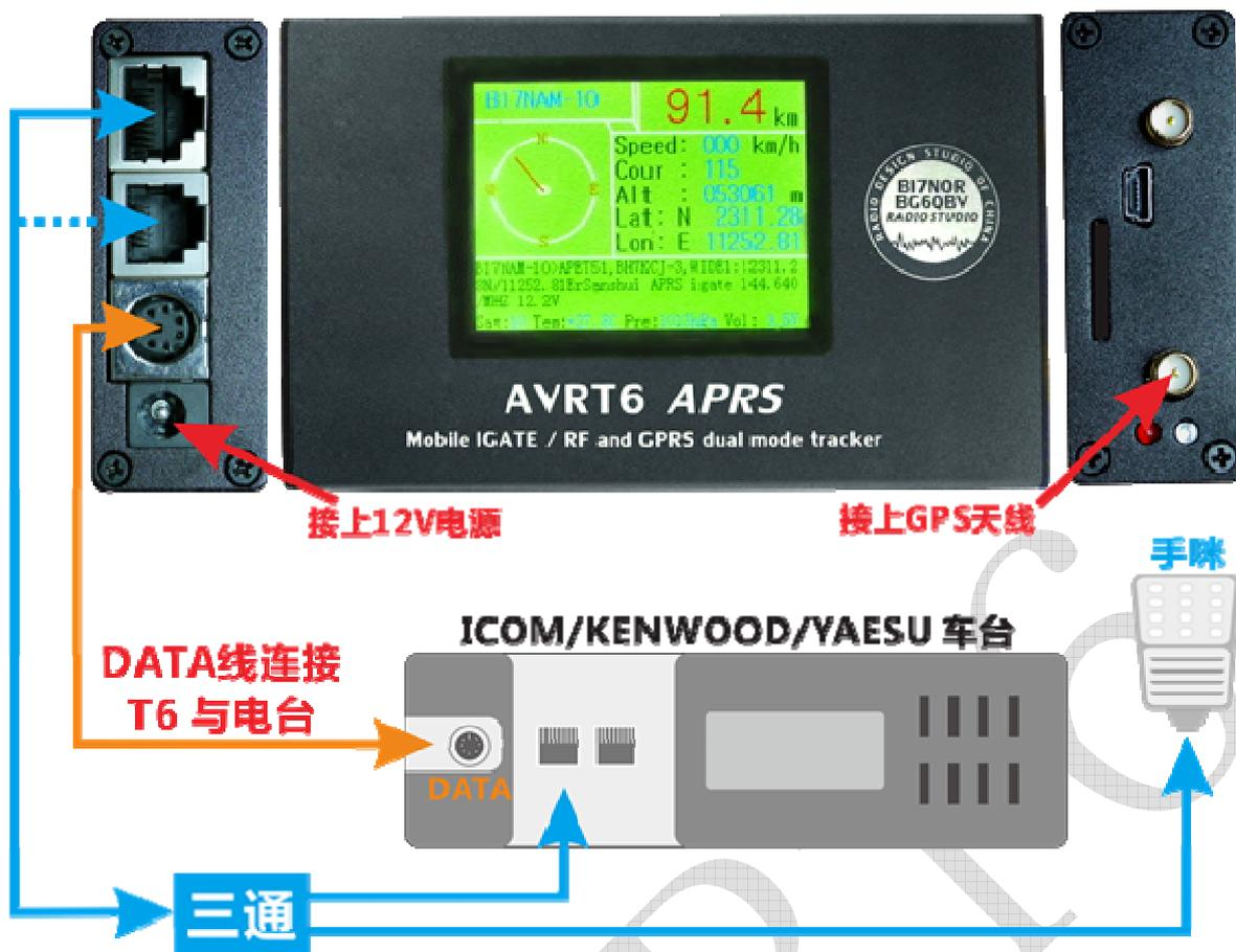
As shown in the figure to connect, without plug SIM card is only RF transceiver, self positioning data, end of contact in the hand microphone PTT moments,T6 launches its own coordinate data by car. GPS positioning, coordinate data that it receives, displays it on the screen and can display real-time data such as distance to each other and call sign, can do communication and positioning without interference.
