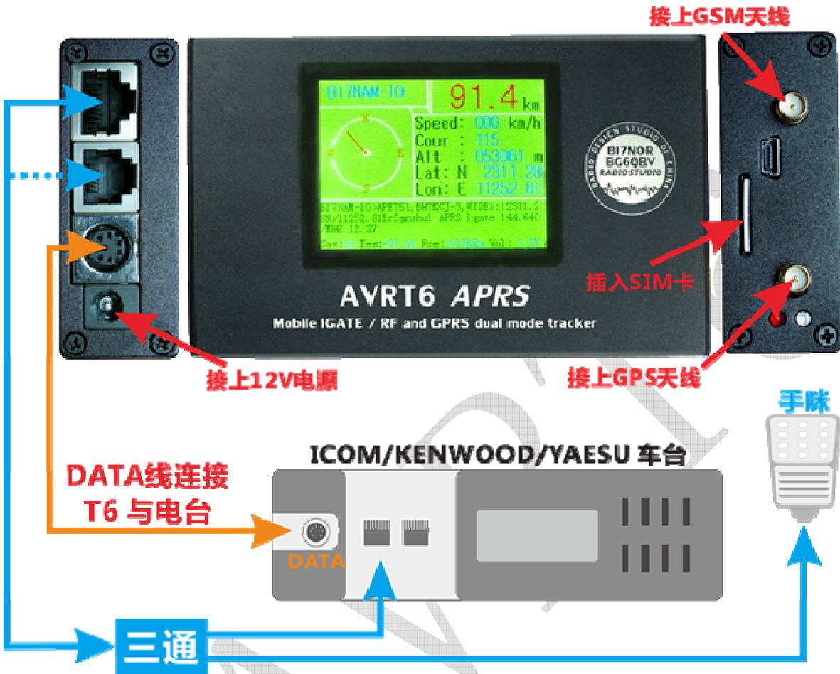
As shown in the figure to connect, compared to the above application is inserted SIM card. This is GPRS+RF double track uploads, and IGATE function, that is, upload gateway.
