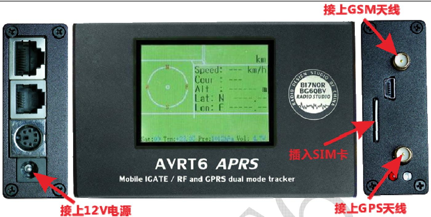
As shown in the figure to connect, insert a valid SIM card is the simplest of GPRS network upload path function. Displays only the data displayed on the next line, shows the number of satellites, the temperature, the pressure and the supply voltage.
